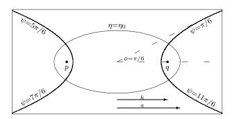
Figure 2: The magnetic field penetrates an elliptical portion of a moving conductor. The level curves of coordinate  $\eta$  are ellipses with foci p and q, a distance 2h apart. The level curves of  $\psi$  are semi-hyperbolae; the value of  $\psi$  is the polar angle of the asymptote. The boundary of the magnetic field is given by  $\eta = \eta_0 = \cosh^{-1}(\frac{1}{\epsilon})$ . The semi-major axis of the boundary is a.
