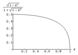
Figure 3: The reduction factor in the current density for an arbitrary ellipse as a function of the ellipse's eccentricity.
