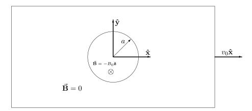
Figure 1: Magnetic field penetrating a circular portion of a moving conductor.
